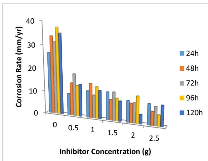
Figure 4: Effect of inhibitor concentration on corrosion rate.
